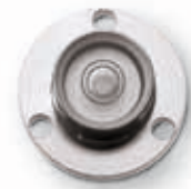
Bullseye vial in aluminium frame, Ø 30 x 11 mm R 1700 mm \pm 4 min. Article N°. 680 030 DFM
