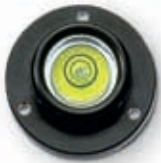
Bullseye vial in plastic frame, Ø 30 x 11 mm R 130 mm \pm 53 min. Article N°. 680 030 DFK
